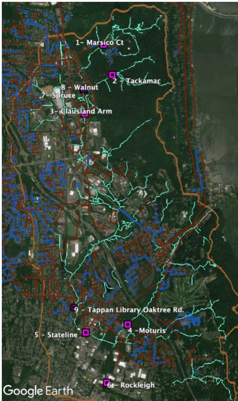
Figure 1: Map of the Sparkill watershed showing surface water in aqua, locations of samples 1-9 (see Table 1) with white labels, stormwater lines in blue and sanitary sewer lines in red.
